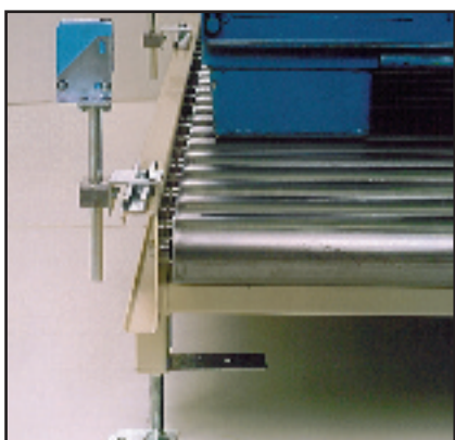
Sensors guarantee an accurate positioning of the goods to be conveyed.
