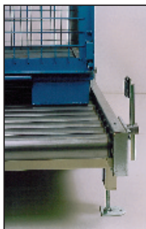
The closed drive side with the sensor reflector.
