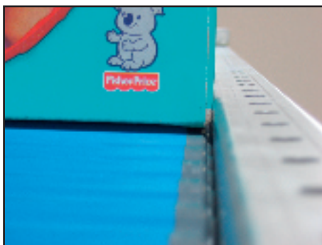
A lateral guiding of 15 mm is created on installation of a bearing roller with a diameter of 30 mm above middle height.
