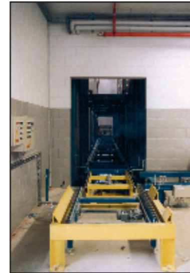
Picking aid for fork lift truck and turnaround station
